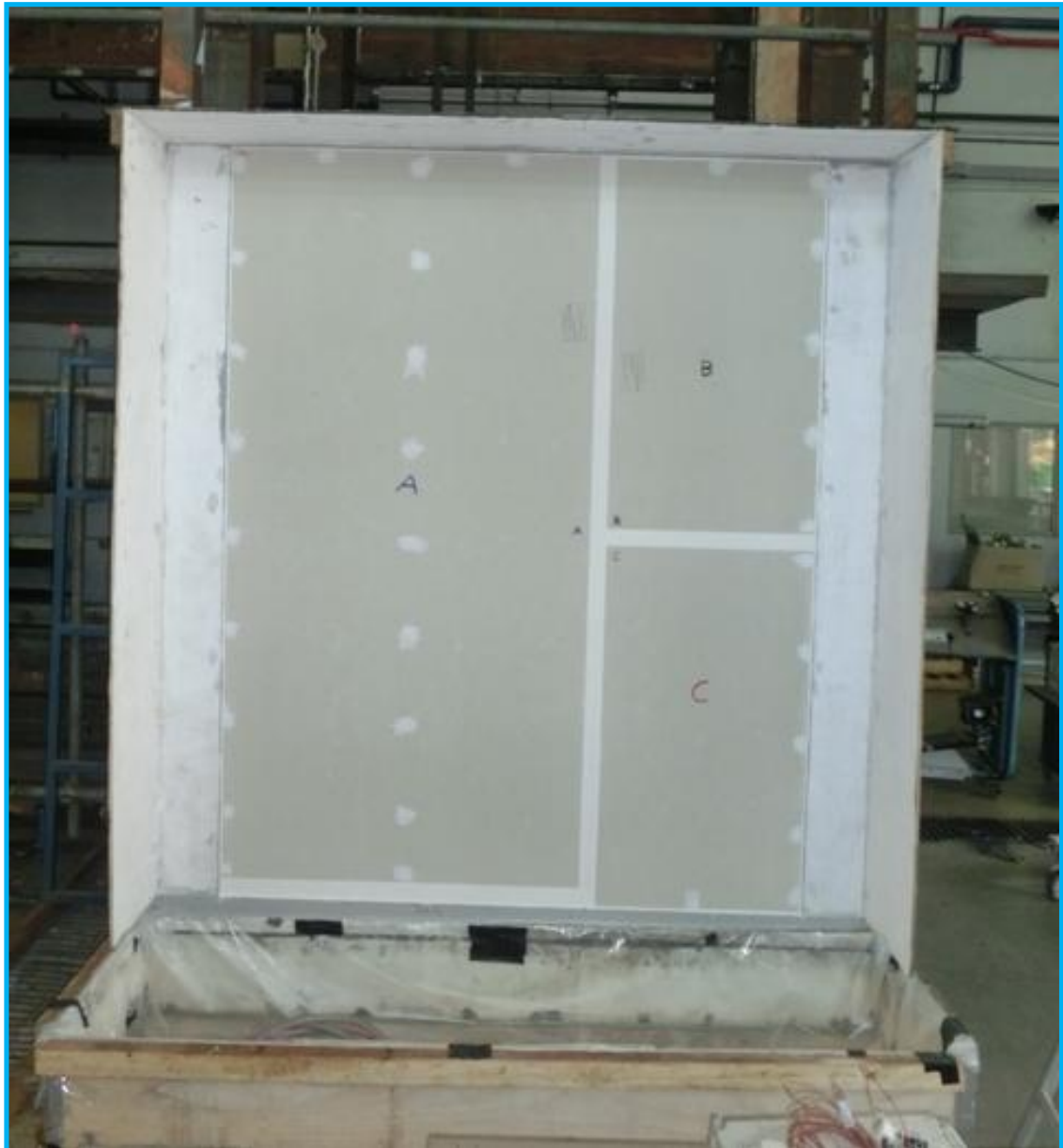
Photo 1: “SCG SmartBoard” Fibre cement board mock-up. (Indicated with alphabet markings for surface observation before and after test)
