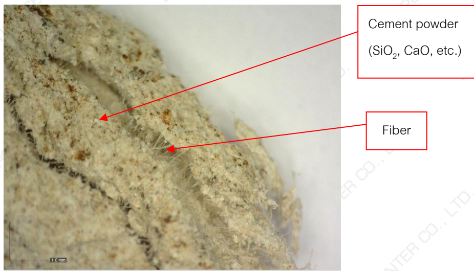
Figure 1 Picture of Smartboard 1200x2400x12 mm by optical microscope
